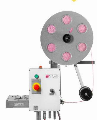
Various plastic thicknesses (in red) handle a wide range of package types, weights and sizes. Closures can be printed with price, date and/or code information. Available colors vary with plastic thickness: .030" - 7 colors .045" - 3 colors > .045" - white only
