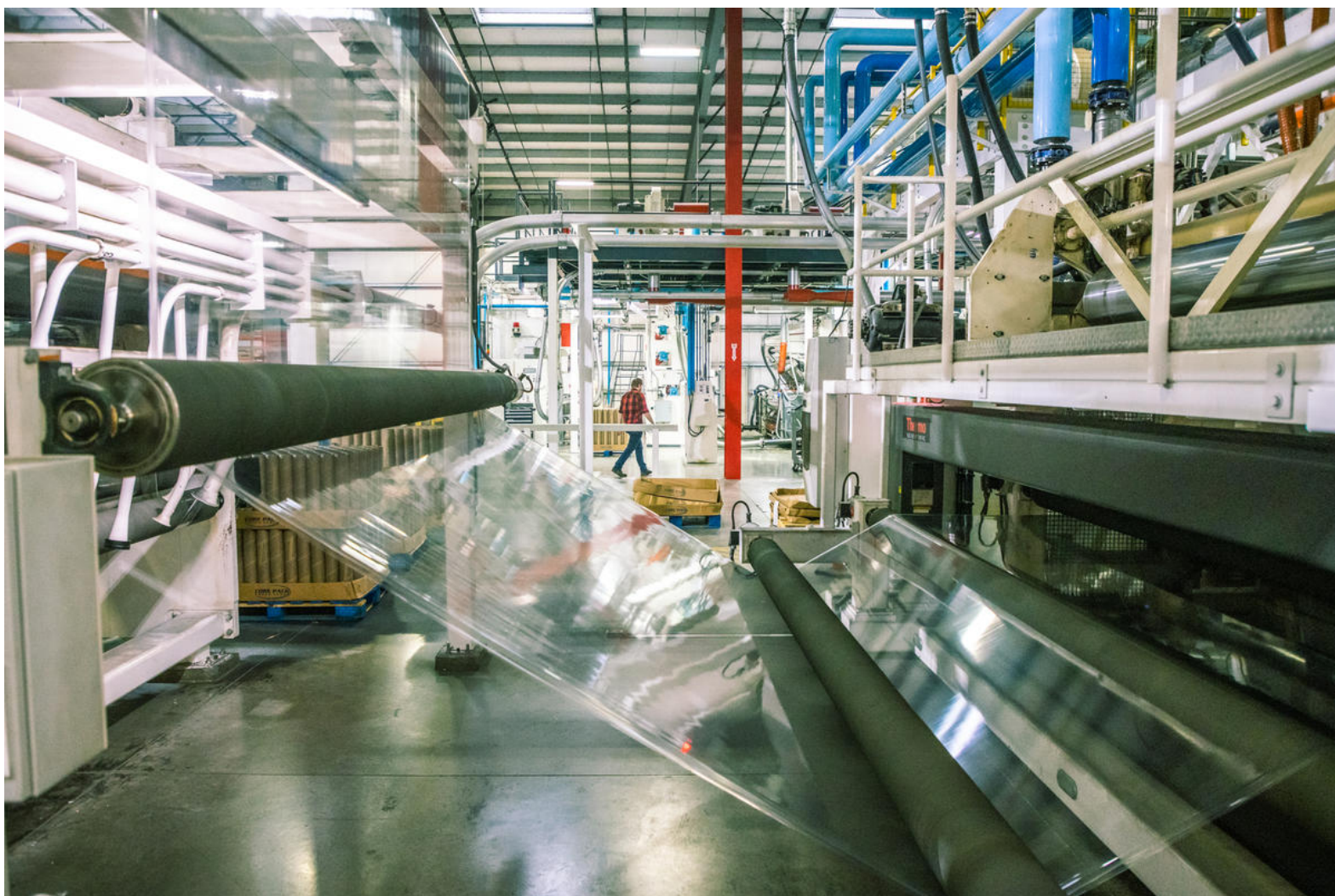
A sheet of Titus handfilm makes its way through the production facility at Paragon Films on Thursday, Nov. 11, 2021 in Union Gap, Wash. Titus is one of Paragon Films’ proprietary stretch film, and is thinner than most other stretch films in its class. This cuts down on material and waste. (Jake Parrish for Crosscut)
